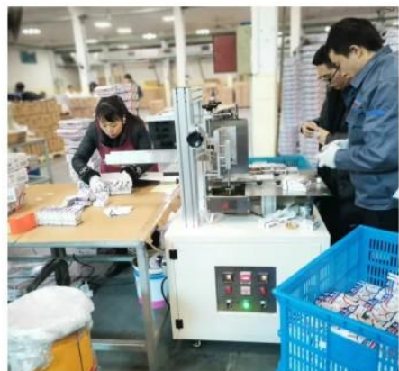
手推式封盒机应用 Application of hand sealing machine
